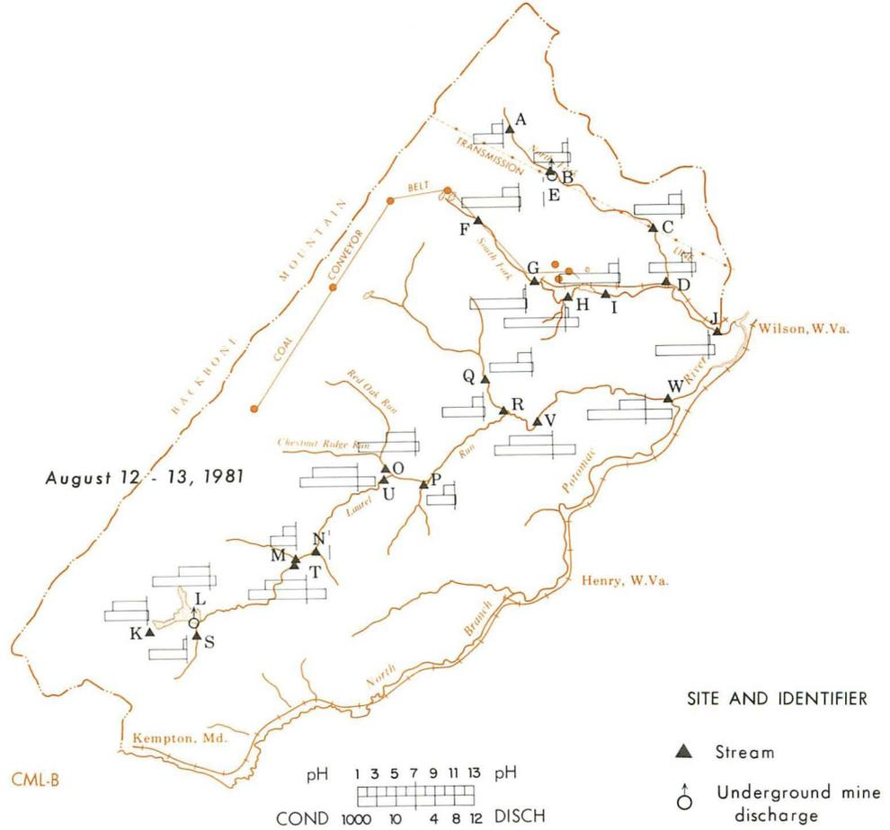
Figure 17.—pH, specific conductance, and discharge at the seepage-investigation sites.
