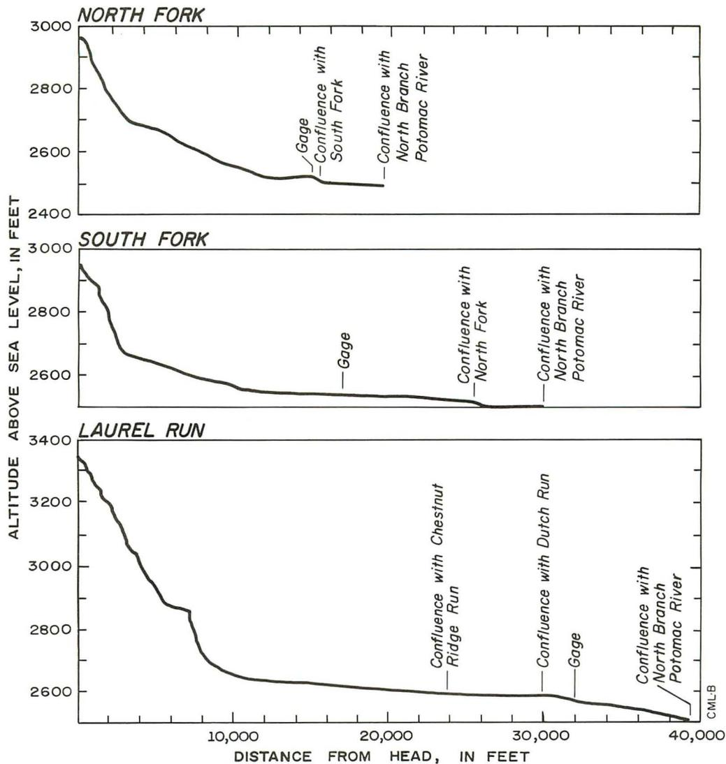
Figure 3.—Channel profiles of North Fork, South Fork, and Laurel Run.
