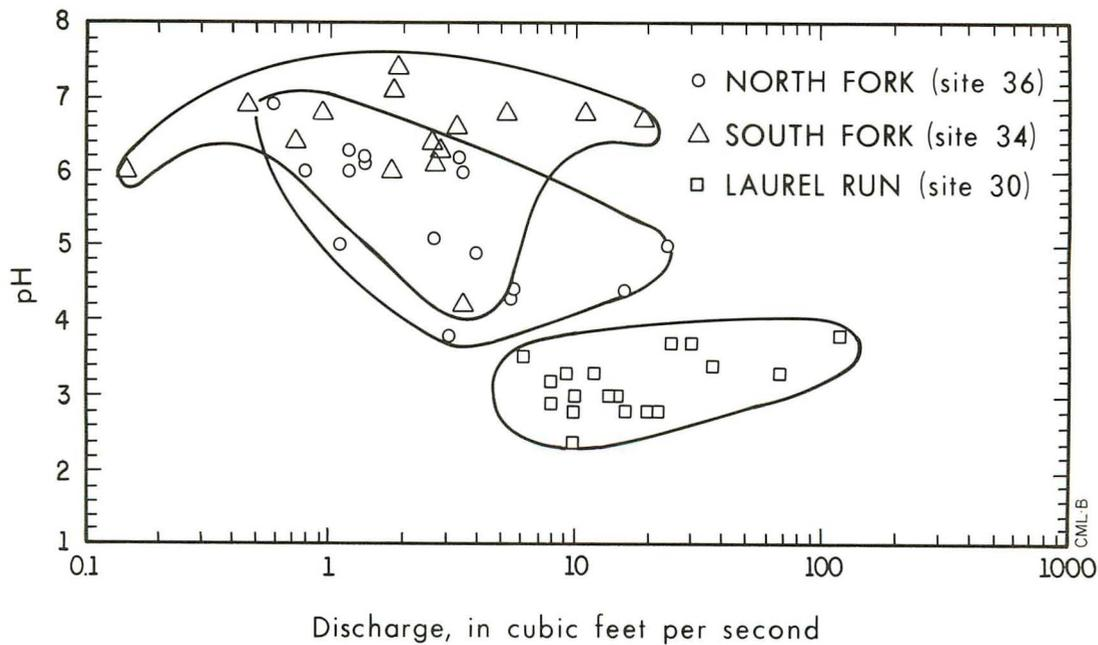
Figure 20.—Relationship of pH and discharge in North Fork, South Fork, and Laurel Run.
