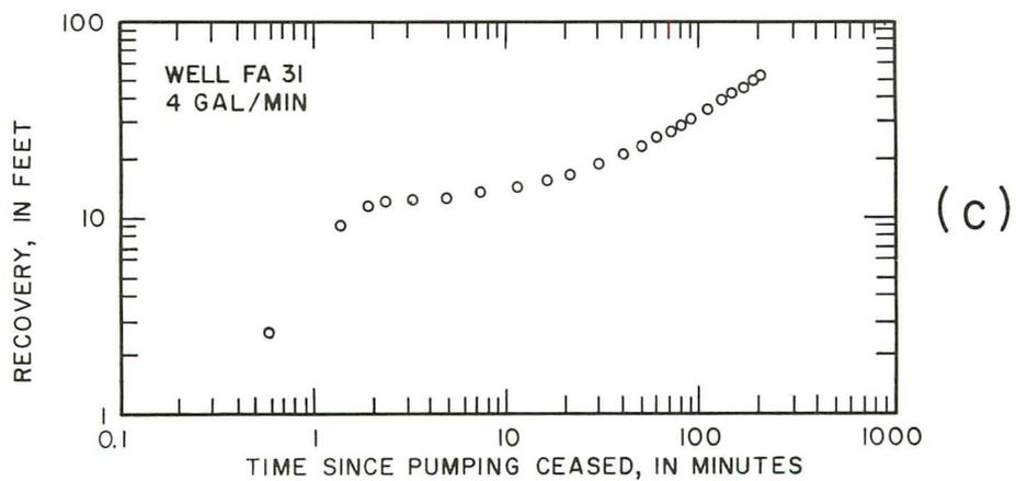
Figure 27.—Examples of drawdown and recovery data for selected wells.
