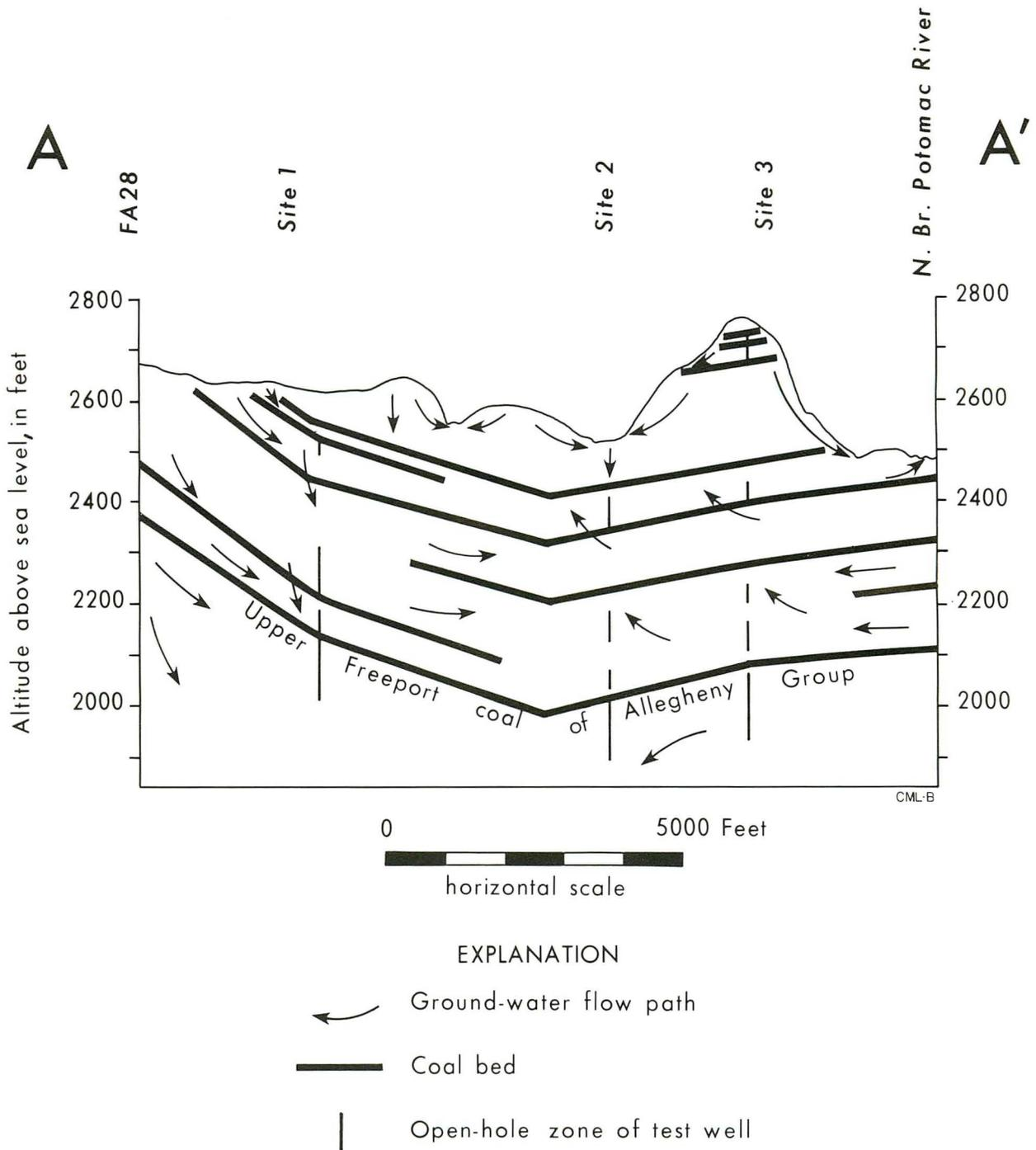
Figure 30.—Possible ground-water flow paths prior to April 1981.
