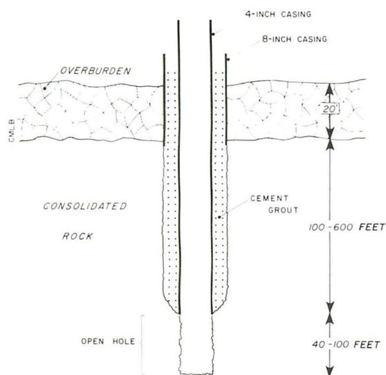
Figure 23.—Typical observation-well construction.
