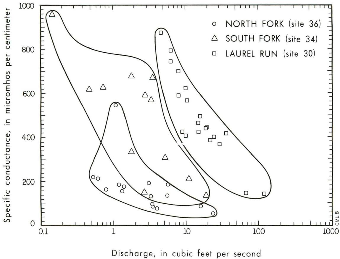
Figure 19.—Relationships of specific conductance and discharge in North Fork, South Fork, and Laurel Run.
