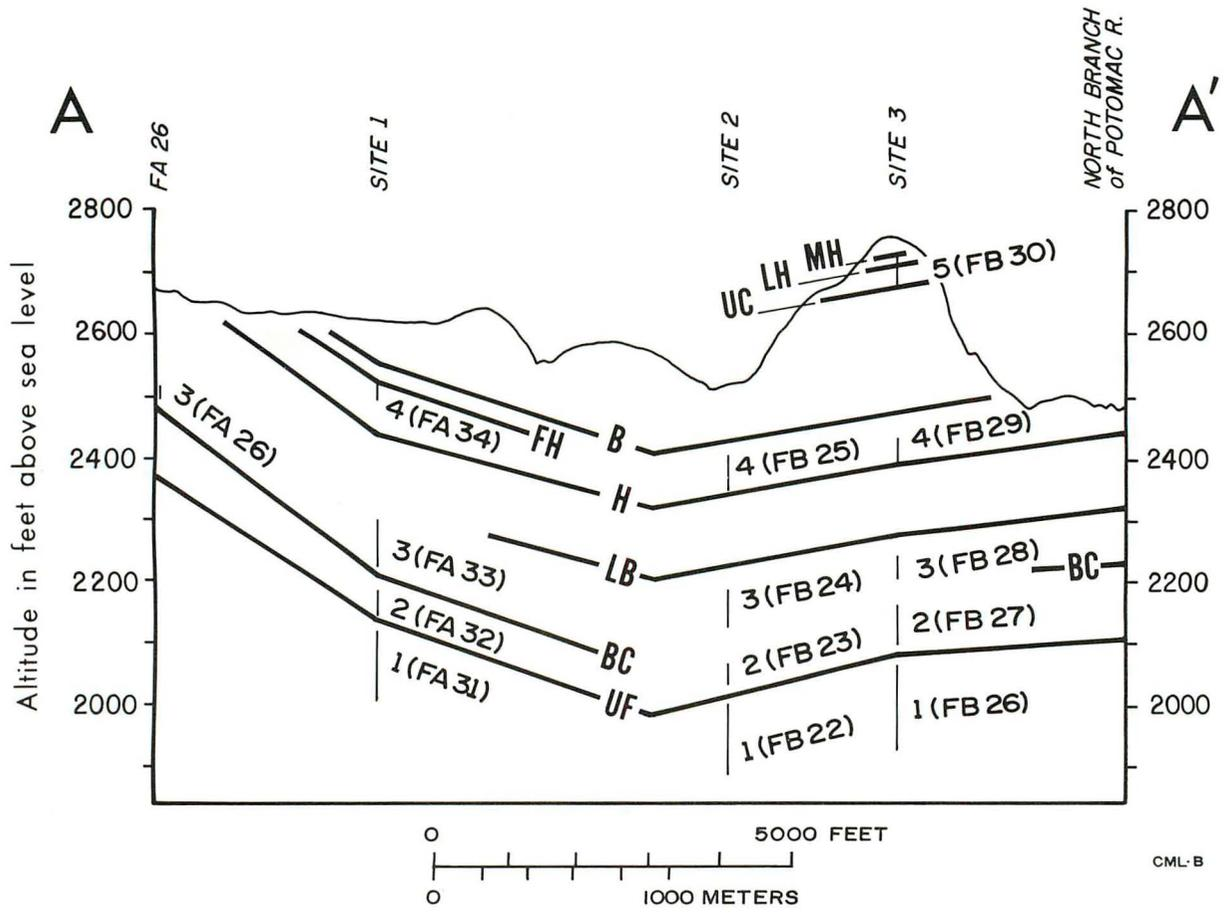
Figure 22.—Open-hole zones of wells and identification of coals.
