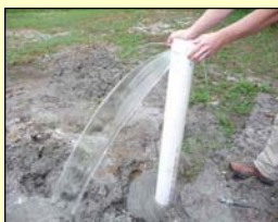
Flowing artesian conditions
