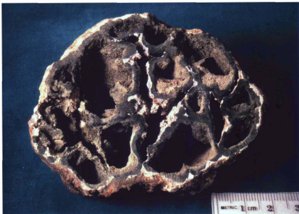
Figure 53: Cross section of a phosphate nodule from the former WWV antenna site, Greenbelt, Maryland. Dark gray (dark green) is mostly lipscombite, light gray (light green) is mostly rockbridgeite, and white (light pink) is phosphosiderite. Specimen is about 9 cm long (NMNH 102572).
