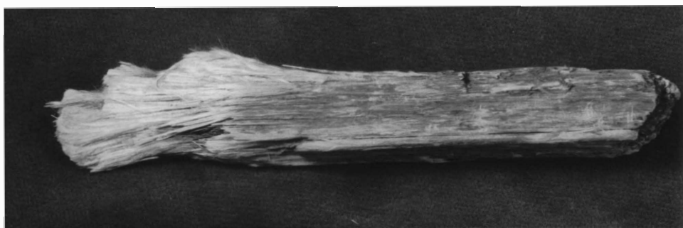
Figure 11: Anthophyllite asbestos from the Bok asbestos mine, Hollofield, Maryland. Specimen is 11 cm long.
