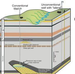
Figure 4. Conventional versus unconventional gas well drilling. In unconventional drilling the source bed becomes the gas reservoir.
