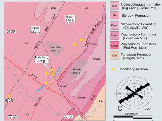
Figure 3. Geologic map of the area surrounding the Albert Powell hatchery (after Brezinski and Bell, 2009 and Brezinski and Fauth, 2009).
